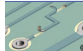
1. Remove damaged conductor.
