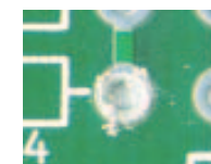
Damaged plated hole.
