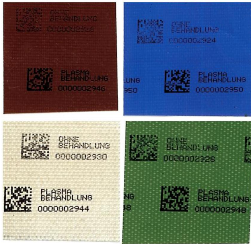
Figure 2: The upper image on each PTFE fabric sample is untreated. There is a clearer, more durable printed image on the bottom of each sample which has been treated.
