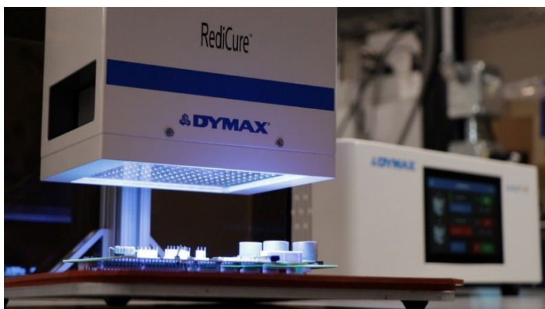
Figure 2 – LED UV curing arrays maintain their intensity for far longer than UV bulbs, enabling more consistent results over time
