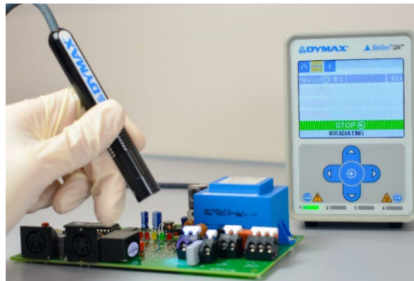
Figure 1 – LED UV curing lamps turn instantly on and off as required during production, drastically reducing energy consumption
