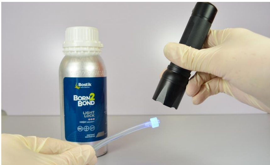
Figure 2 – Dual curing cyanoacrylate adhesives can be considered if parts of the bondline are not visible
