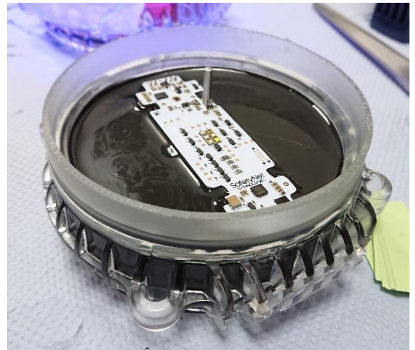
Electronics potting process using IRS 3071
