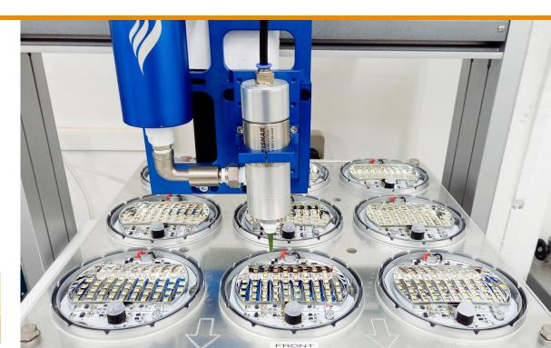
process. They came to us for help in improving the quality of dispense and overall repeatability. The **Fisnar ADVANCE robot** we recommended, along with a **CR300 cartridge retainer** and **HP790 dispensing valve**, allows them to de-skill the process and semi-automate it. The result is a more accurate dispensing method which produces reliable, high-quality products."
