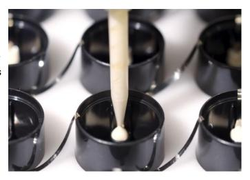
After working with DD-Scientific to understand the details of its application, Intertronics recommended and supplied several **preeflow® eco-DUO precision metering, mixing and dispensing systems**, and integrated them with **Fisnar dispensing robots**. The two-component precision volumetric, positive displacement system uses a progressive cavity pump principle to achieve an accuracy of ±1%, >99% of the time.
