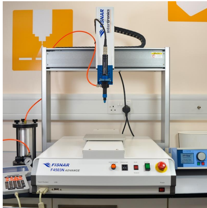
Figure 6 – Dispensing accuracy and repeatability can be significantly improved with automated, robotically controlled processes
