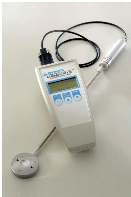
Figure 4 – A radiometer should be used to regularly check the intensity of the UV curing lamp
