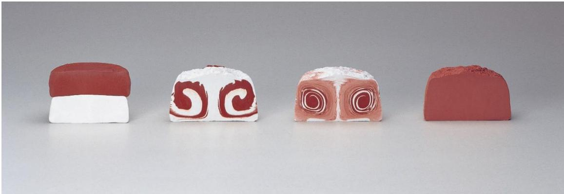
*Example of modelling clay which has been mixed using the planetary principle.*
