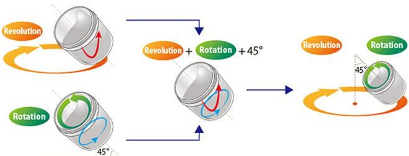
The technology results in a fast, fully homogeneous mix and, unlike machines that rely on the insertion of paddles or impellers into the material, no air is introduced; in fact, the shear forces finely disperse any entrapped air, and there is a tendency for it to be removed (“squeezed out” to the surface).
