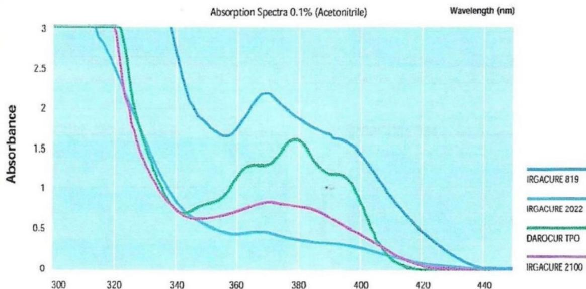
Figure 3 – Absorption spectra of some Ciba photoinitiators (0.1 wt % in acetonitrile solvent)<sup>2</sup>
