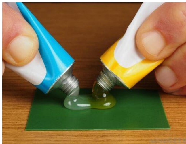
Figure 2 – Working life for two-part systems like epoxies will be an important selection factor
