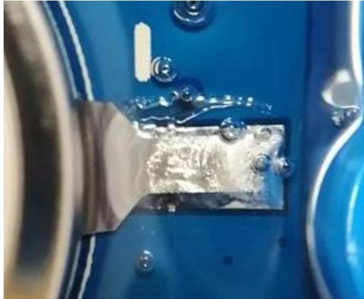
*Figure 8 – Moisture on the surface of the PCB assembly caused CO<sub>2</sub> bubbles to form in the polyurethane potting compound*
