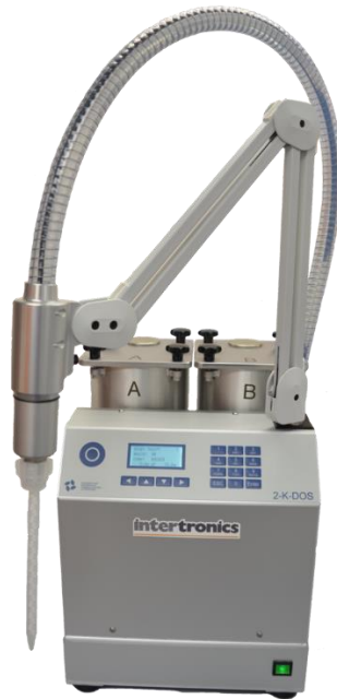
Figure 4 – A dedicated metering, mixing and dispensing machine will prepare materials without entrapping air (2-K-DOS Metering, Mixing and Dispensing System)
