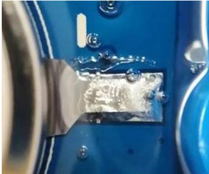
Figure 8 – Moisture on the surface of the PCB assembly caused CO 2 bubbles to form in the polyurethane potting compound
