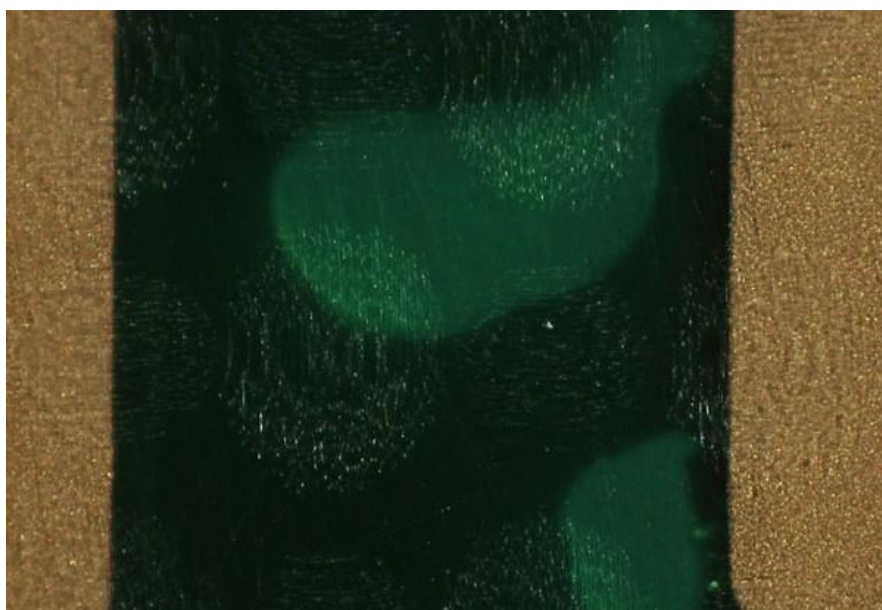
Figure 1 – Grinding away the layers, almost completely through the PCB, uncovers two copper tracks, and in the centre, the remaining solder resist. Under the resist, some voids in the potting compound are apparent.
