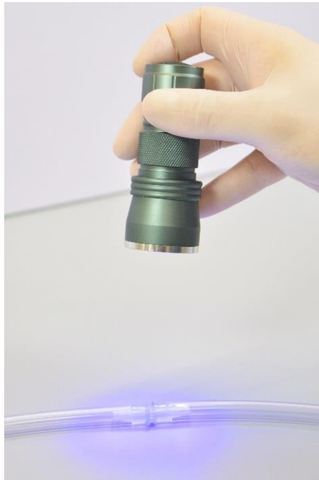
Figure 3 – A low powered UV torch can be used to cure exposed fillets of Born2Bond Light Lock cyanoacrylate adhesive.
