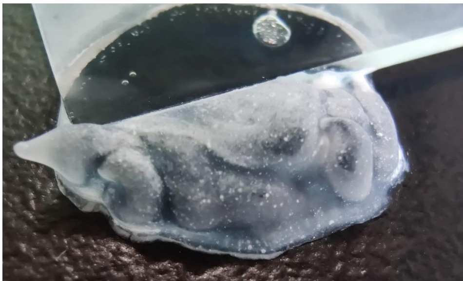
Figure 1 – Example of blooming or frosting formed on an exposed fillet of cyanoacrylate adhesive
