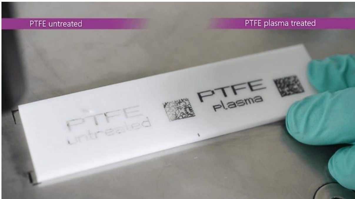
Figure 5 - Adhesion test of inkjet printing on untreated and plasma-treated PTFE
