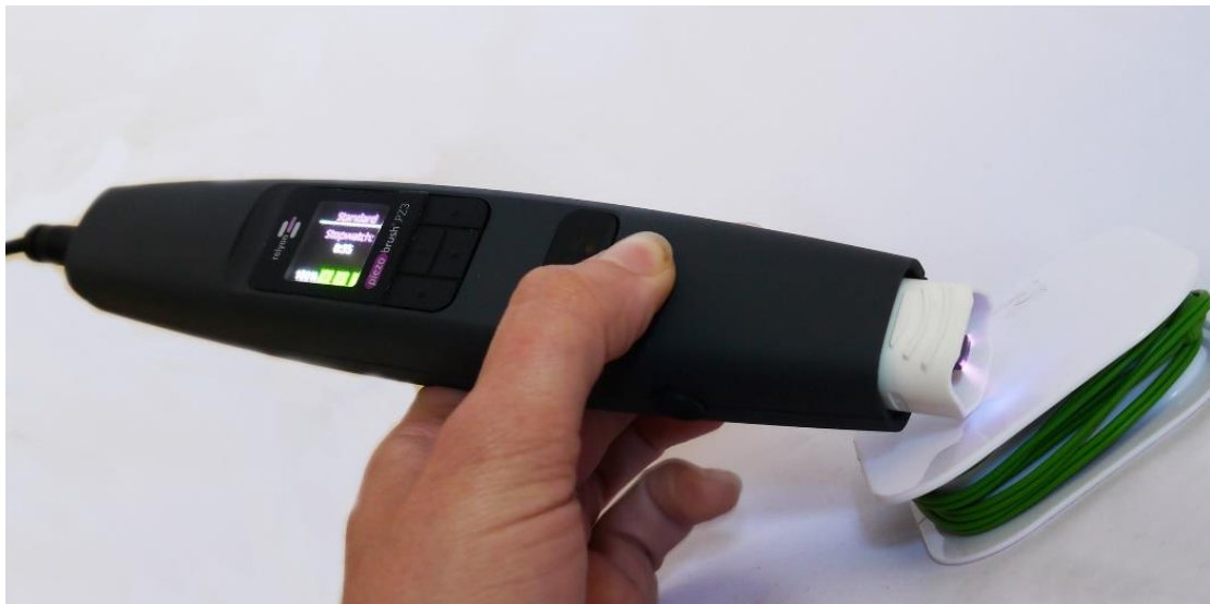
Figure 1 – piezobrush PZ3 treating ABS substrate
