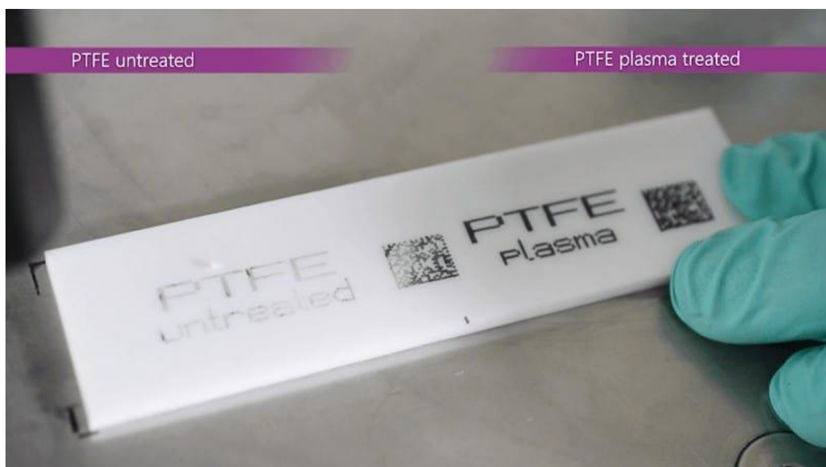
Figure 5 - Adhesion test of inkjet printing on untreated and plasma-treated PTFE
