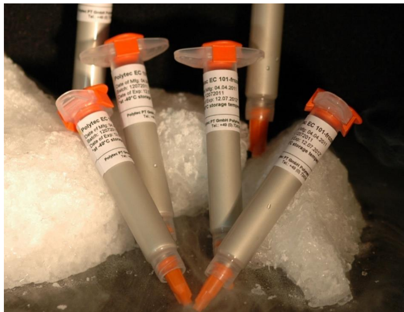
Figure 1 – Pre-mixed and frozen two-part adhesives supplied in syringes
