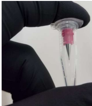
Image is a nozzle hub lodged inside lid of packing tube
