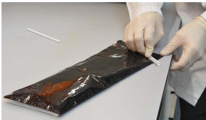
The lightweight filler can separate from the resin before mixing.
