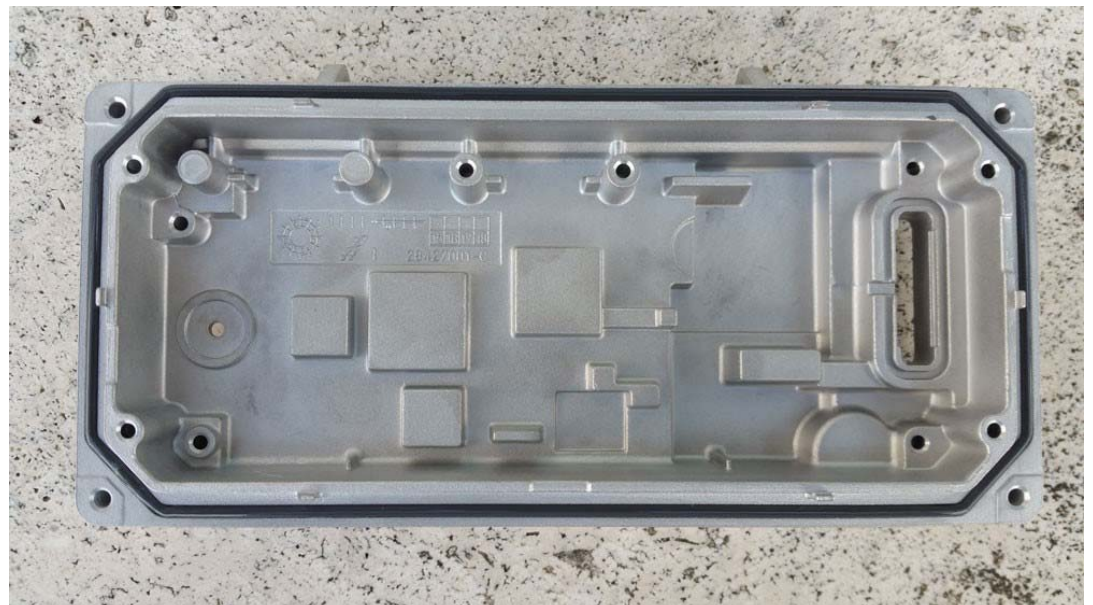
Completed material application with even material join
