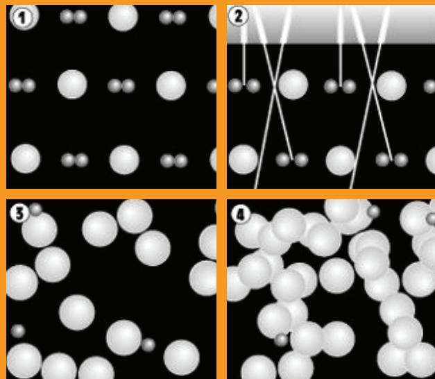
With most UV curing adhesives (i.e. those based on free radical polymerisation), curing starts with exposure to light, and stops when the light is removed. So, the production process should ensure a full cure during the time of exposure. If possible, expose all adhesive in one dose of UV light. Multiple exposures are not normally recommended as they could affect the integrity of the bond.
