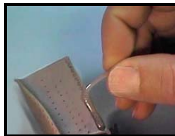
Figure 8. Removal of a Peelable Masking Resin
