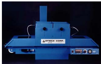
Figure 6. Conveyor with Overhead Curing Lamps
