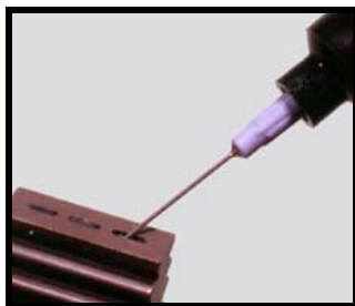
Figure 7. Core filling with a Burn-Off Masking Resin
