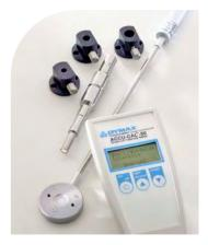
Dymax offers the ACCU-CAL<sup>™</sup> 50 radiometer which measures UVA (320-395 nm) light for spot lamps, floods, and conveyors. The ability to measure light intensity is useful for three reasons:
