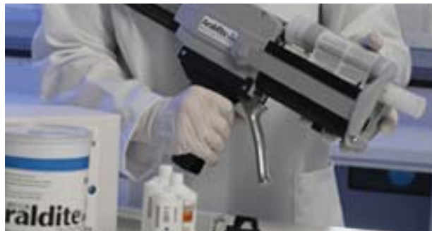
Fit resin & hardener cartridges into dispensing gun
