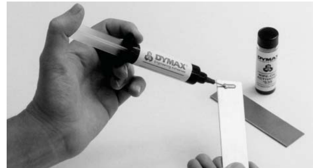
Apply adhesive to other surface
