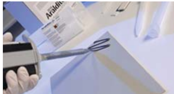
Squeeze trigger to dispense mixed media
