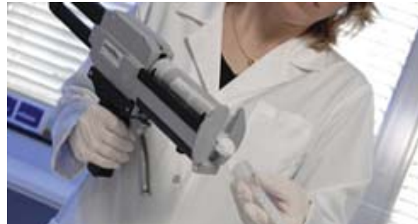
Attach recommended mixing nozzle to gun
