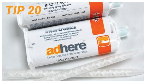
Many two part adhesives are packaged in side-by-side double syringe cartridges; the adhesive is dispensed through a static mixing nozzle. Before attaching the nozzle, always gently squeeze the dispensing gun trigger and make sure that both of the material components are being pushed out evenly. Wipe off any excess material, and then screw on the static mixing nozzle.
