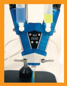
Metering, mixing and dispensing machines are useful for the automation and control of higher volume two-part systems. For the most part, these machines are specific to a particular material.
