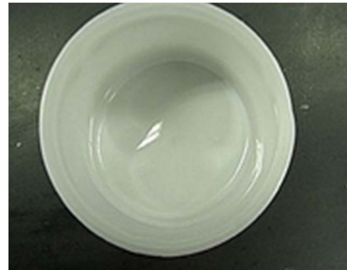
Mixing talc into a viscous silicone
