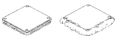
Figure 7 - Encapsulation of QFP leads for security reasons
