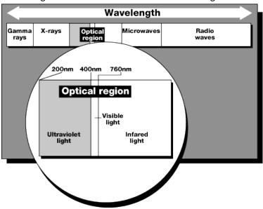
Figure 1 - The Electromagnetic Spectrum
