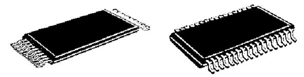
Figure 6 - TSOP surface mount components, Type I and Type II
