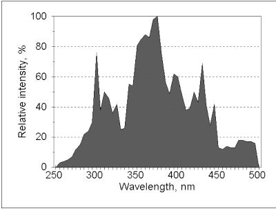
Figure 3 - Relative Spectral Output of Curing Lamp
