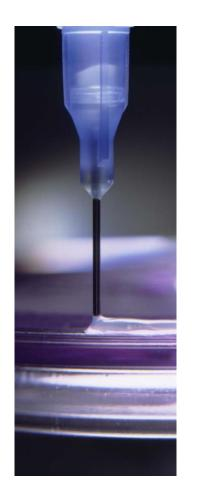
The use of adhesives to provide a structural bond can take the place of mechanical fasteners – and provide advantages to your business, including performance and reliability improvements, and reduction in manufacturing costs.
