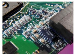
Clear Conformal Coating on PCB
