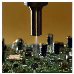
Conformal Coating Sprayed on PCB
