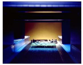
Conformal Coating Curing in Conveyor System
