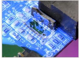
Cured Dual-Cure Coating Under PCB Component
