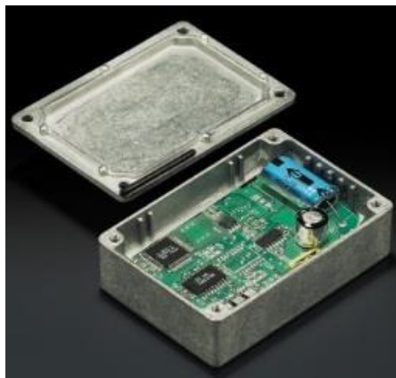
Figure 2 - Opti-tec 7020 is a clear silicone potting compound
