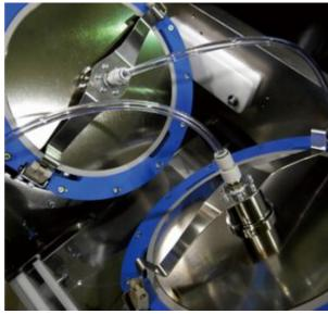
Simultaneous mixing and deaeration of up to 20L of material
