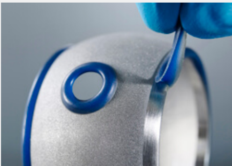
DYMAX SpeedMask is removed
