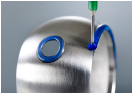
DYMAX SpeedMask is applied
