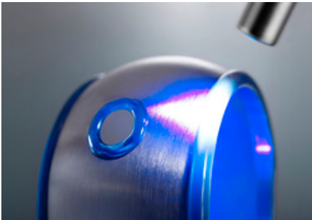
Dymax SpeedMask is UV cured instantly
