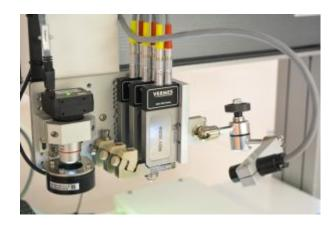
A camera vision system is incorporated to allow for easier, more accurate programming using fiducial marks to provide exact control over dispensing placement.
