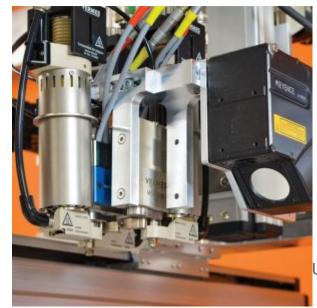
Ultra-precise contactless dispensing of a hot melt
