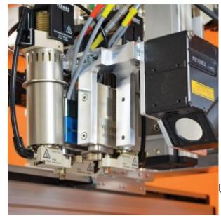
Ultra-precise contactless dispensing of a hot melt
