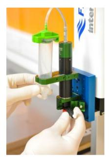
This semi-automated adhesive dispensing system was assembled for a customer who was applying pre-mixed and frozen electrically conductive adhesives to sample parts for mass spectrometry. These adhesives can be difficult to dispense if they begin to cure quickly, leading to blockages in the dispensing valve or needle if there is any production downtime.
