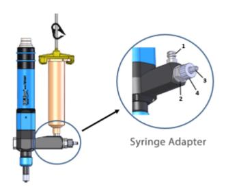
Made of black anodized aluminium and stainless steel, and FFKM sealing elements, the syringe adapter is compatible with almost all materials and allows for air bubble-free dispensing, even after several syringe barrel changes.
