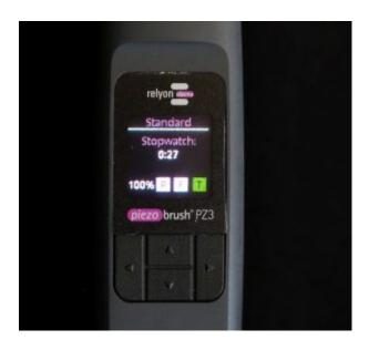
For process control of plasma treatment, the PiezoBrush PZ3 is equipped with various features that can be selected and modified via the user friendly display.
