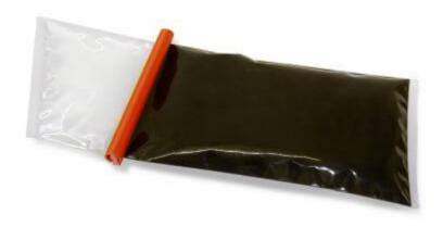
The twinpack sachet is a clear film sachet, with the resin and hardener separated by a removable clip and rail divider. Click here for twinpack mixing instructions.
