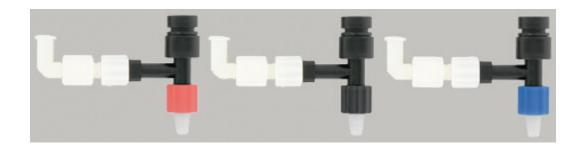
The valve allows for easy maintenance and is suitable for abrasive materials and two-part fluids, solder pastes and SMD adhesives. It has a short fluid path with no dead space, minimising material wastage. The **IDMVG DV5005DFS Positive Displacement Auger Valve** delivers precise, repeatable dots and beads for any automated or manually operated application.
