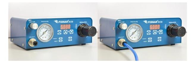
As standard, the DC50 dispensing controller releases regulated, compressed air through its built-in male push connector fitting. 6mm (1/4") tubing can be easily hooked-up to the controller, with no additional components required.
