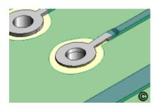
5. Complete connection to the conductor
