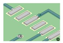
5. Complete connection to existing conductor
