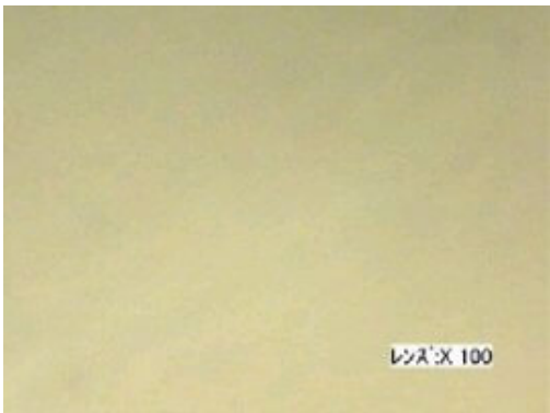
After curing – 100x magnification (2000rpm @ 0.7kPa for 5 minutes)
