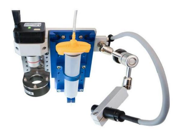
The Robot Vision System comprises two cameras, including one for live dispensing images
