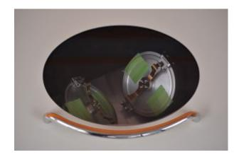
The **THINKY ARV-931Twin Mixer** has two degassing/defoaming modes as standard features: one is vacuum deaeration mode which combines 400G centrifugal force and vacuum, and the other is atmospheric pressure deaeration mode which utilises powerful centrifugal force of maximum 670G. This enables high precision degassing even with materials that contain a volatile component that is not suitable for vacuum deaeration.
