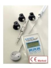
**ACCU-CAL 50-LED UV Intensity Meter**
