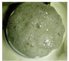
Caution must be taken to prevent foaming and messy overflows when manually degassing using vacuum
