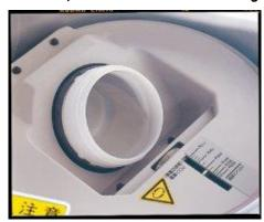
Materials don't overflow because they are pressed to the side wall of the container during the simultaneous mixing procedure
