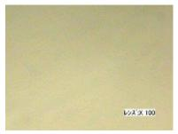
No bubbles are observed in cured resin 100x magnification
