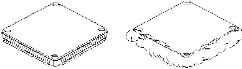
Figure 7 - Encapsulation of QFP leads for security reasons
