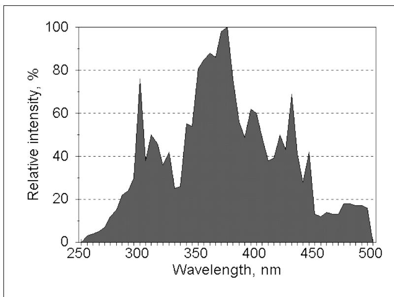
Figure 3 - Relative Spectral Output of Curing Lamp
