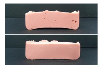
Air entrapment from manual mixing (above) can be mitigated by mixing in a Thinky mixing machine (below)
