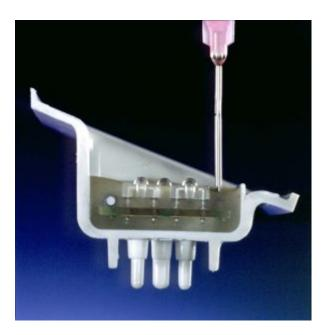
Once your compounds are mixed, it is important not to introduce or entrap air during application. Techniques to eliminate or minimise air bubbles in the completed assembly include pouring or injecting in stages, driving out air rather than trapping it under components. Tilting the assembly, filling from the bottom and perhaps preheating to reduce viscosity and surface tension can help.
