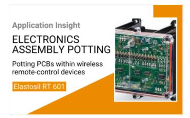
When a manufacturer of wireless remote control devices was looking for a way to pot electronic components on an FR4 circuit board into a moulded clear polycarbonate enclosure, it opted for Wacker <u>Elastosil RT 601</u>. This material is an optically clear, low viscosity silicone potting compound that offers temperature resistance from -40°C to 130°C in both indoor and outdoor environments.
