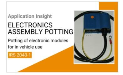
A manufacturer of electronic modules for automotive applications opted for Intertronics <u>IRS 2040-1</u> <u>Epoxy Potting Compound</u> to pot an FR4 board and its electronic components to ABS moulding. Its aim was to protect sensitive electronics from a harsh environment near the engine.
