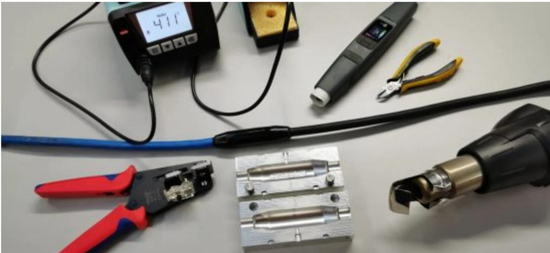
Overmoulding is used to form a watertight and strong mechanical seal around cables used in harsh environments. Wavecon's overmoulding process can involve a wide range of materials depending on the application, including polyethylene, chlorinated polyethylene (CPE), polyurethane, rubbers, and neoprene. Because many of these materials have low surface energies, it causes poor wettability and bonding, creating an adhesion challenge. To improve adhesion, Wavecon had tried abrading the
