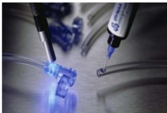
Figure 1 – UV curable adhesives can significantly reduce assembly processing time and costs
